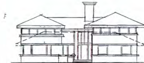
The Contemporary Alteration approach used in putting on a second storey addition.
